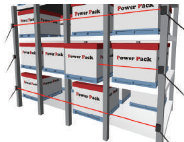
Detecting boxes protruding from shelves (Through-beam type)
